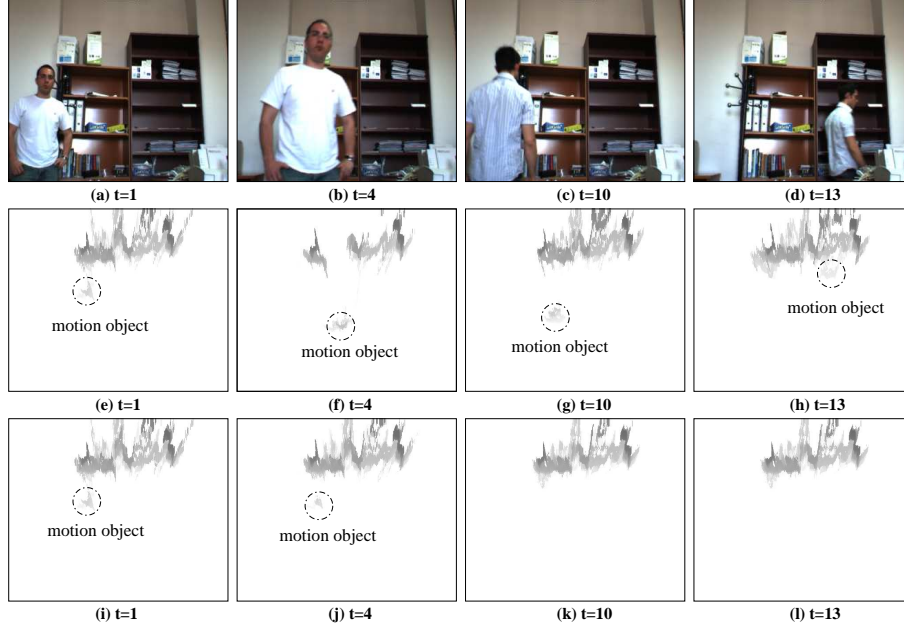
Fig. 2. Creation of the height map. Upper row (a,b,c,d) shows the images in instants 1, 4, 10 and 13. Central row (e,f,g,h) shows the instantaneous height maps \mathcal{H}_{max}^t for each one of the upper images. Lower row (i,j,k,l) shows the evolution of the height map \mathcal{H}_{max} created as the median of the height maps \mathcal{H}_{max}^t created until that moment
