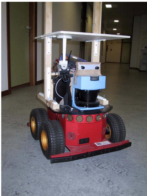
Fig. 2. A Pioneer II AT robot equipped with a laser range scanner.
