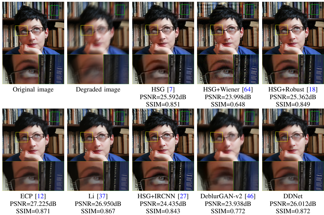
Fig. 4. Visual comparison of the proposed DDNet and competing methods on an image of the Lai [63] spatially invariant degraded dataset.
