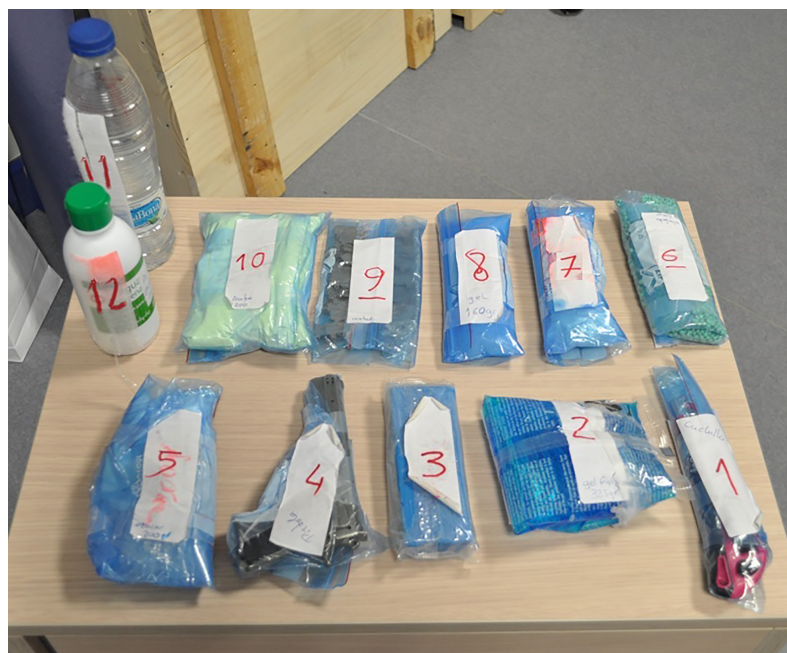
Fig. 8: Simulated threats in the dataset: a cutter (1), 325g of gel (2), a 200g clay bar (3), a simulated gun (4), 200g of sugar (5), 200g of frozen peas (6), 150ml of cologne (7), 160g of gel (8), a bag with metal pieces (9), 200g of flour (10), a 50cl water bottle (11), and a 250ml hydrogen peroxide bottle (12).
