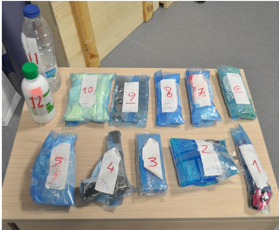
Fig. 13: Simulated threats in the dataset: a cutter (1), 325g of gel (2), a 200g clay bar (3), a simulated gun (4), 200g of sugar (5), 200g of frozen peas (6), 150ml of cologne (7), 160g of gel (8), a bag with metal pieces (9), 200g of flour (10), a 50cl water bottle (11), and a 250ml hydrogen peroxide bottle (12).
