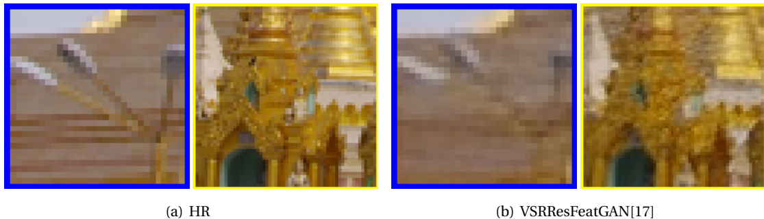
Fig. 3: Examples of artifacts produced by VSRResFeatGAN[17] for scale factor 3. Notice the high frequency artifacts on smooth areas of the image. With the introduction in the loss function of the spatial smoothness constraint term these artifacts are considerably reduced.
