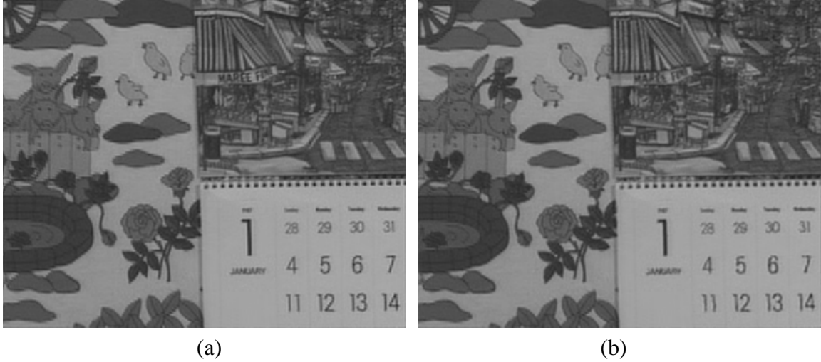
Fig. 5. (a) High resolution estimate with a threshold of 255 for the DFD defined in (17). (b) High resolution estimate with a threshold of 15 in (17). The compressed low resolution motion compensated images \{ \mathbf{m}_l \} are not taken into account in the observation model.
