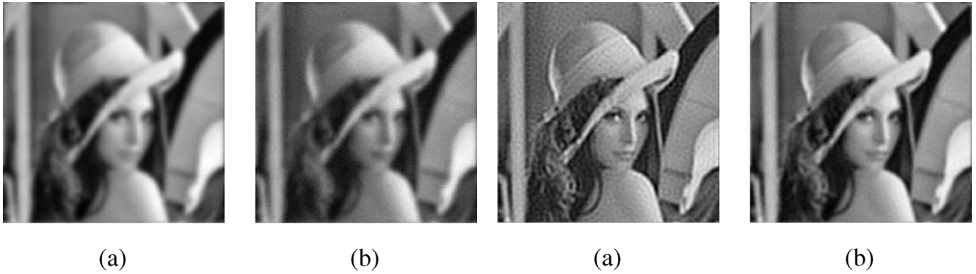
Fig. 1. Images degraded by a Gaussian shaped PSF with variance 9 and Gaussian noise of variance (a) 0.23 (SNR = 40 dB), (b) 16 (SNR = 20 dB).
