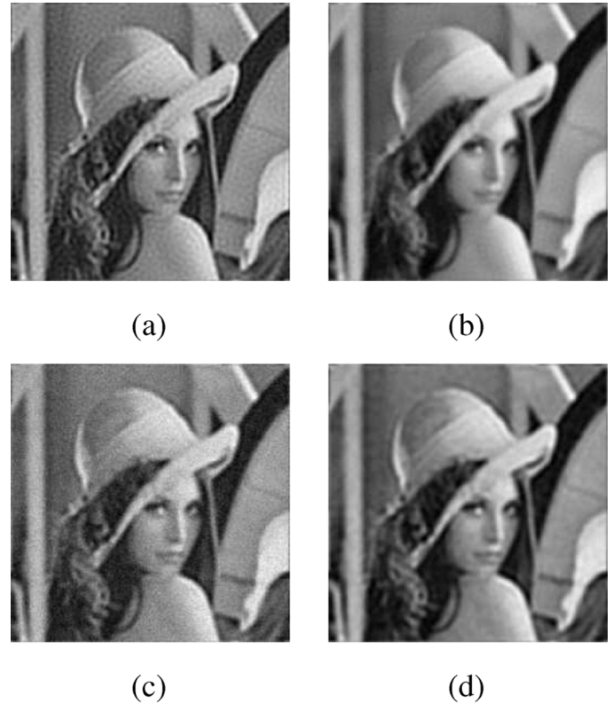
Fig. 2. Restorations of 40-dB SNR Lena image using (a) the MOL method, (b) the LG method, (c) the BR method with \gamma_{\omega} = 0 , \omega \in \{\alpha_{im}, \alpha_{bl}, \beta\} , and (d) the BD method with \gamma_{\omega} = 0 , \omega \in \{\alpha_{im}, \alpha_{bl}, \beta\} .
