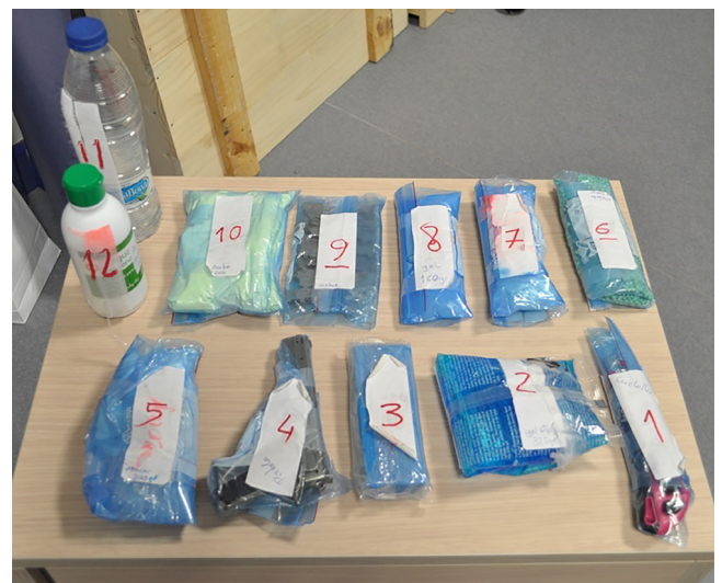
Fig. A.8. Simulated threats in the dataset: a cutter (1), 325 g of gel (2), a 200 g clay bar (3), a simulated gun (4), 200 g of sugar (5), 200 g of frozen peas (6), 150 ml of cologne (7), 160 g of gel (8), a bag with metal pieces (9), 200 g of flour (10), a 50cl water bottle (11), and a 250 ml hydrogen peroxide bottle (12).
