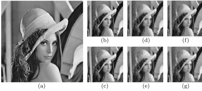
Fig. 5. Reconstruction of LR images. (a) Lena original HR image, (b, c) Downsampled images Q = 2 , P = 2 , Blur Var = 3, R = 0.8 , SNR = 30 dB, (d, e) First estimates of the LR images, PSNR = 40.22 dB and 40.16 dB, respectively, (f, g) Final estimates of the LR images, PSNR = 42.88 dB and 42.77 dB, respectively.
