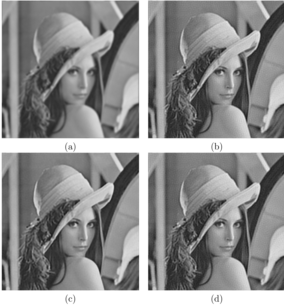
Figure 2: (a) Observed Lena image for gauss blur at 30 dB; (b) Restoration using SAR method; (c) Restoration using \ell_1 method; (d) Restoration using the proposed method for \lambda_1 = 0.3 .
