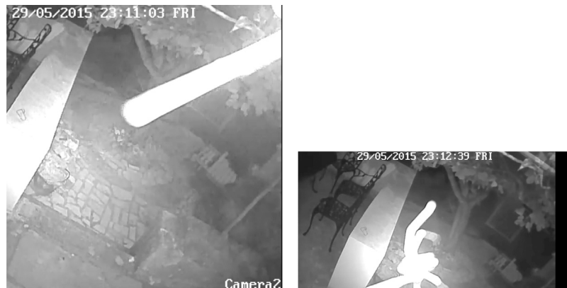
Fig. 9. Two examples of night vision camera. White areas corresponds to a spider weaving his web.
