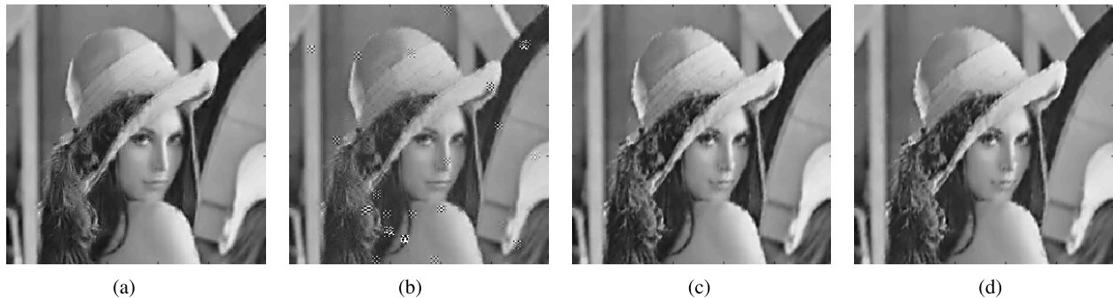
Fig. 5. Comparison of the inpainting performances at r = 75\% of BKSVD, K-SVD [60], BPFA [30] and Spike and Slab (SnS) model [35] algorithms. Please note that in this comparison the dictionary is learnt from the corrupted images themselves. (a) BKSVD inpainting. (b) K-SVD inpainting. (c) BPFA inpainting. (d) SnS inpainting.
