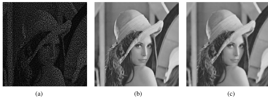
Fig. 4. Comparison of the inpainting performance of BKSVD and K-SVD algorithms. Please note that in this comparison the dictionary is learn from a set of clean images. (a) r=75\% missing pixels. (b) BKSVD inpainting. (c) K-SVD inpainting.
