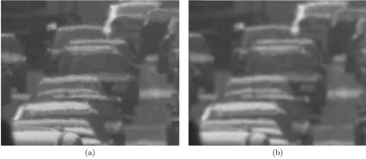
Figure 3. Cropped 13 frame of the “Rush-hour” sequence. (a) high resolution frame of the sequence coded at 2 Mbps (PSNR = 36.06 dB). (b) Super resolved frame from the sequence coded at 1 Mbps (PSNR = 36.56 dB). Similar visual quality is achieved with a 50% reduction of the bitrate.
