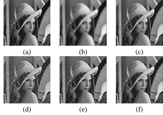
Fig. 1. (a) Original “Lena” image, (b) Degraded image, (c) Restoration by MLE method. Restorations for (d) BR approximation with \gamma_\omega = 0.0 , \omega \in \Omega , (e) BD approximation for \gamma_\beta = 1.0 , \gamma_{\alpha_{im}} = 1.0 and \gamma_{\alpha_{bl}} = 0.8 , and (f) BR approximation for \gamma_\beta = 1.0 , \gamma_{\alpha_{im}} = 0.5 and \gamma_{\alpha_{bl}} = 1.0 .
