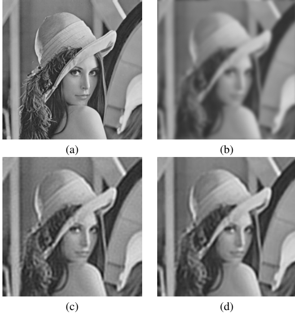
Fig. 2. (a) Original Lena Image, (b) Image degraded by a Gaussian shaped PSF with variance 9 and Gaussian noise of variance 0.16 (BSNR=40dB), (c) Restored image using Algorithm 1 with p = 1.8 (ISNR = 4.15dB), (d) Restored image using Algorithm 2 with p = 1.6 (ISNR = 3.78dB).
