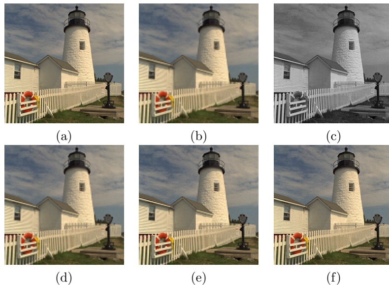
Fig. 2. (a) Original HR color image; (b) Observed LR color image (the image has been resized by zero-order hold to the size of the high resolution image for displaying purposes); (c) Panchromatic HR image; (d) Bicubic interpolation of (b); (e) Reconstruction using the global image model proposed in Ref. 8; (f) Reconstruction using the local image model proposed in Ref. 10.
