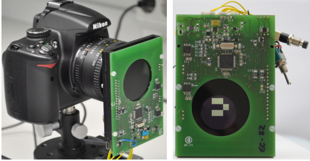
Fig. 1. (a) Mechanical interface, electronic control board and LCD, mounted in the prototype. It is equipped on a Nikon D5000 camera with a Nikkor 50mm f/1.8 lens. (b) The LCD showing one of the coded apertures.
