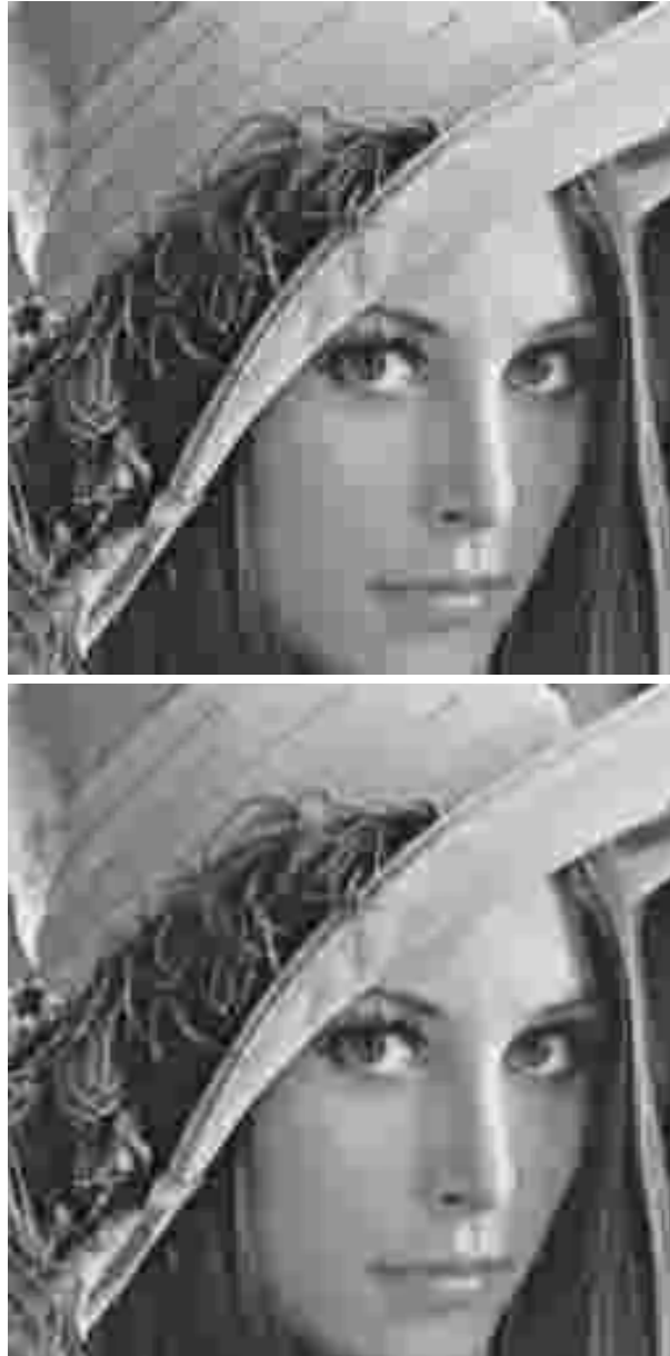
Figure 1.3 256 \times 256 center section of "Lena": (top) JPEG based compression at 0.22 bpp, PSNR = 29.58 dB; (bottom) reconstruction, hyperparameters estimated at the decoder, PSNR = 30.16 dB.
