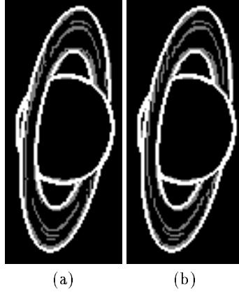
Fig. 4. Comparison between the real edges (light) and the obtained line process (dark). (a) Proposed ICM method, (b) Proposed SA method
