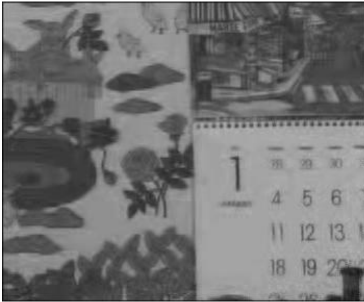
Figure 8. Result of the Non-Synthetic Experiment with Nine Frames. The compression rate is 256 kbps, and the PSNR is 29.5dB.
